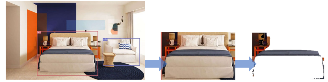
Figure 5. During the process, beds are detected and cropped from the image and then patterns are segmented from beds.
